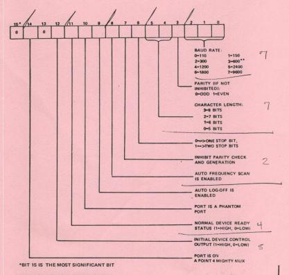
\*\* ON A POINT 4 MUX WITH THE 19200 BAUD OPTION, 3=19200, NOT 600
