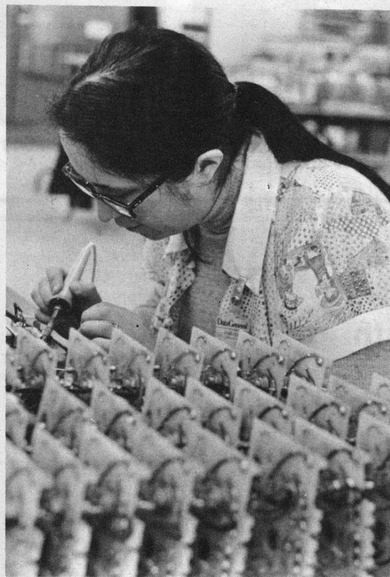
LINING 'EM UP - Jolene Trefethen applies her hand soldering talent to power/fail boards.
