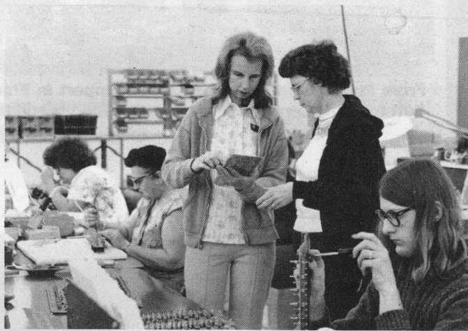
CHECKING IT OUT - Heleana Foster (standing with board) and Ferieda Whitney double check their work as (left to right) Pam Clemons, Rose Raitt and Barbara Pray perform hand soldering and touch-up operations.
