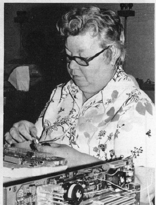
PRE-SCREENING - Kay Burnett inspects components that will be part of a front console panel.
