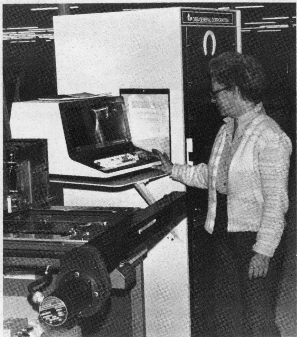
PUNCHING UP COMPONENTS - Dottie Ostrowski activates this Data General designed automatic component insertion machine with a simple entry into a Data General CRT.
