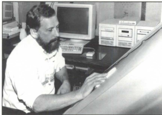
GIS specialist Brad Kincaid uses digitizer to enter map into GIS data base.
