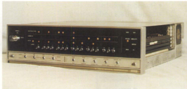
Original Nova, #262, still running with 4KW core memory
