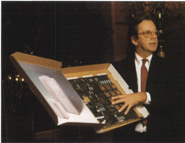
J. Tom West, senior vice president Advanced Systems Development, talks to the press. He holds a sample of the quad-processor board that fits in a pizza box.
