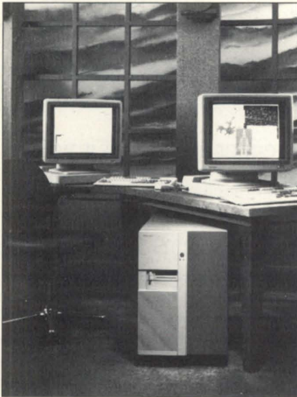
Data General's new 88000-based family of industry-standard products includes the 88000-based system (below table) and personal workstations with 19-inch monochrome and 20-inch color displays.
