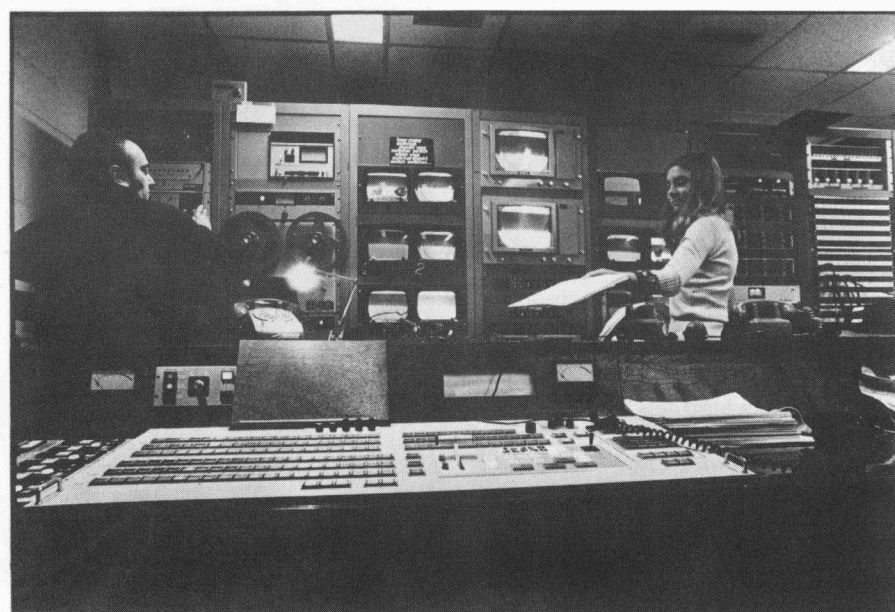
In the control room of Channel 38 in Boston, a traffic clerk delivers the station's daily log, produced by an intelligent terminal built around a Data General Nova 2/10 computer. The terminal is part of a system offered by Data Communications Corporation of Memphis and now in use at over 100 radio and television stations in the United States. It keeps track of advertising schedules and rates and generates the daily log.
